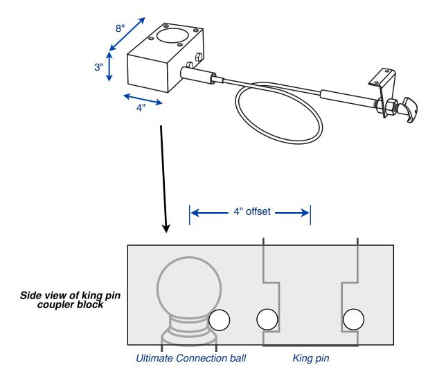
NOTE: The above king pin coupler is included with Part # 3200 (rail mount), 3225 (gooseneck mount) and 3235 (extended gooseneck mount)
